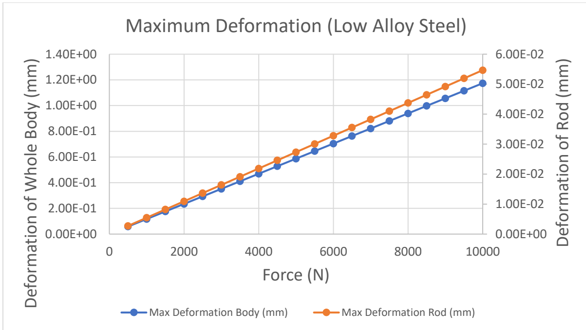
Figure 37: Maximum deformation experienced by the whole body and the rod for loading conditions of 0-10000N (low alloy steel)
