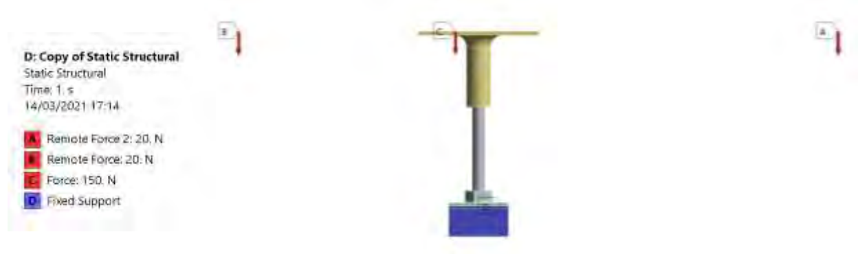
Figure 25: Boundary conditions of bending loading
