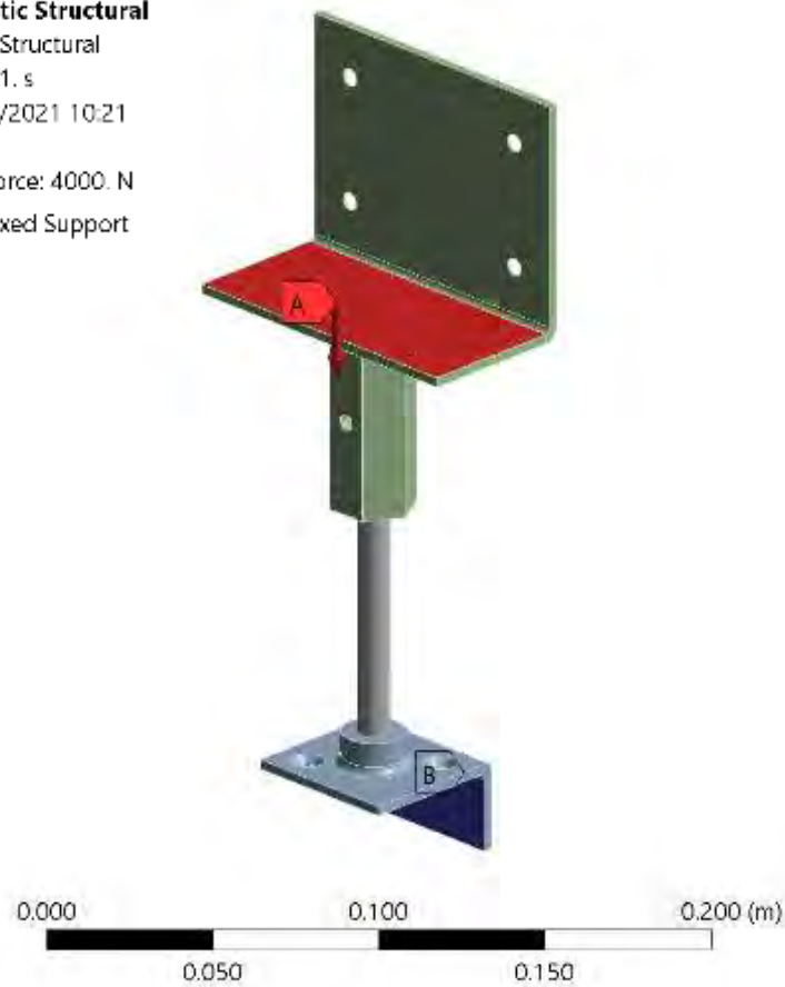
Figure 9: Boundary conditions applied to structure
